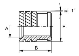
Female thread A = M3,5 Length B = 6.3 Min distance to edge = 2.5 Outer diameter E = 5.00 Recommended bore diameter = 4.6
